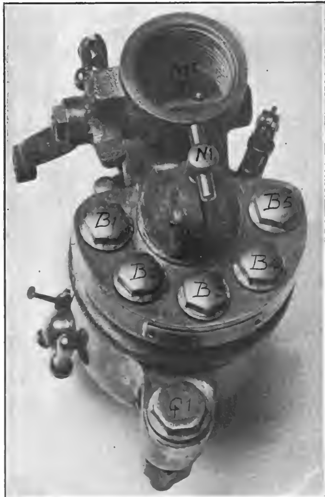
Fig. 8—Looking down upon the carbureter, showing the orifice for connecting the intake manifold and the caps covering the floating balls
